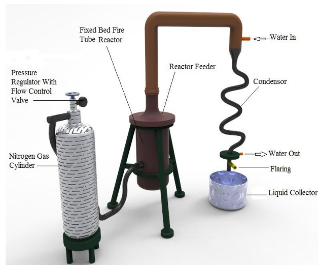
Fig.1: Shows the schematic view of the experimental set-up
